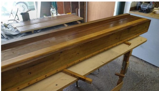
The refurbished pedal wind chest. The pipes sit inside this organ
